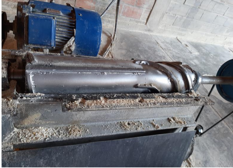
Locally made maize degerminator
